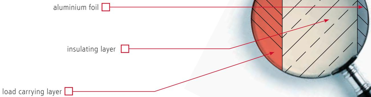
Fig. 2 Cross-section of the curtain's coat
